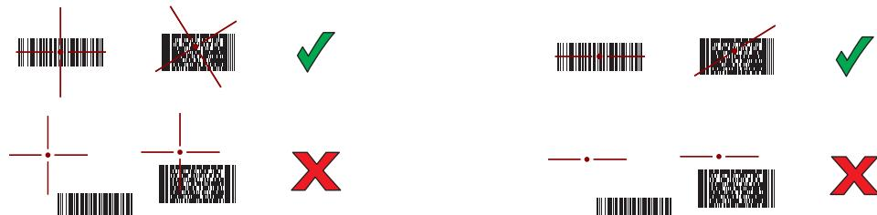
Figure 29 Pick List Mode with Multiple Barcodes in Aiming Pattern: Standard and Extended Range
