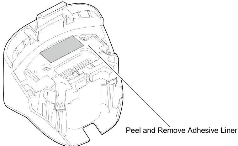
3. Insert the adapter into the MC9XXX cradle and adhere to the bottom of the cradle.
