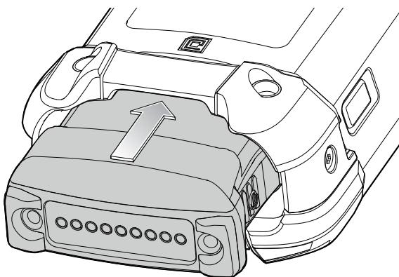
2. Push the battery into the battery slot.
