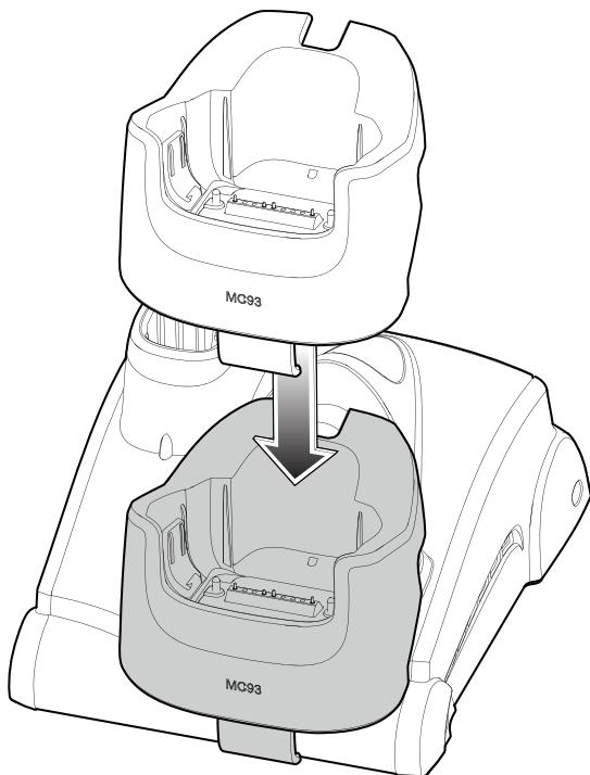
4. Insert the device into the cradle.
