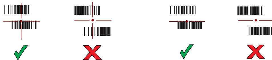
5. Release the Scan button or trigger.
