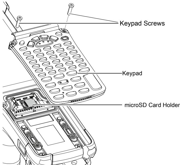
7. Lift the keypad from the device.
