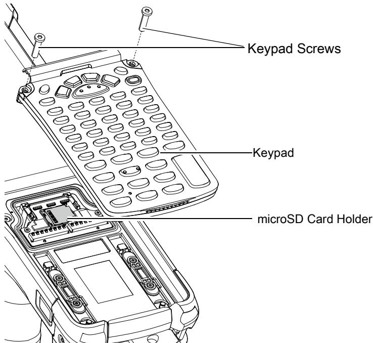
7. Lift the keypad from the device.
