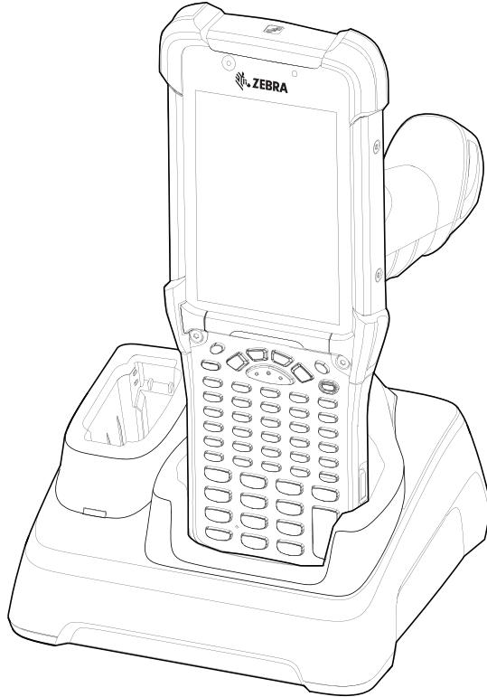
3. Gently press down on the device to ensure proper contact.
