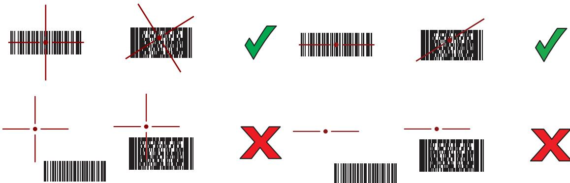
Figure 79 Pick List Mode with Multiple Barcodes in Aiming Pattern: Standard and Extended Range
