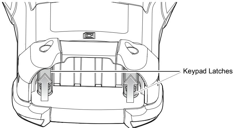
16. Using a Torx T8 screwdriver, replace the two keypad latch screws inside the battery slot and torque to 5.8 kgf-cm or 5.0 lbf-in.
