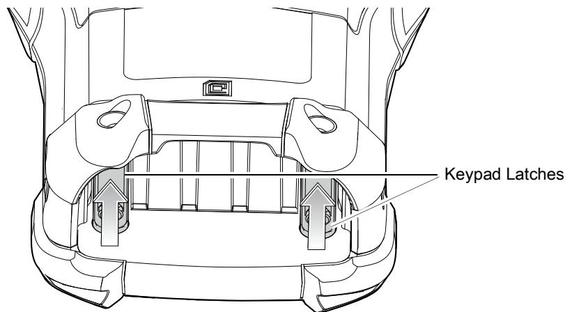
12. Using a Torx T8 screwdriver, replace the two keypad latch screws inside the battery slot and torque to 5.8 kgf-cm or 5.0 lbf-in.
