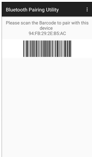
2. Using the RS507/RS507X or RS6000, scan the barcode on the screen.
