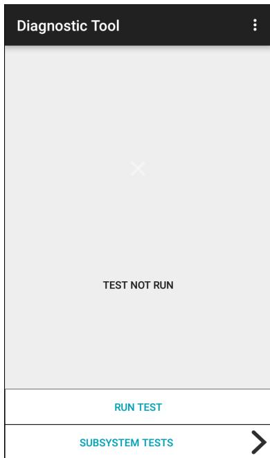
2. Touch **RUN TEST**. The app tests all enabled subsystems (by default, only the Battery and System tests). See Settings to enable subsystem tests.
