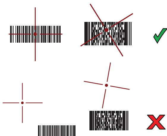
Figure 87 RS6000 Pick List Mode with Multiple Barcodes in Aiming Pattern
