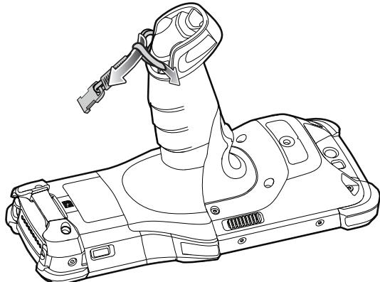
2. Thread and pull-through the longer section through the opening near the battery.
