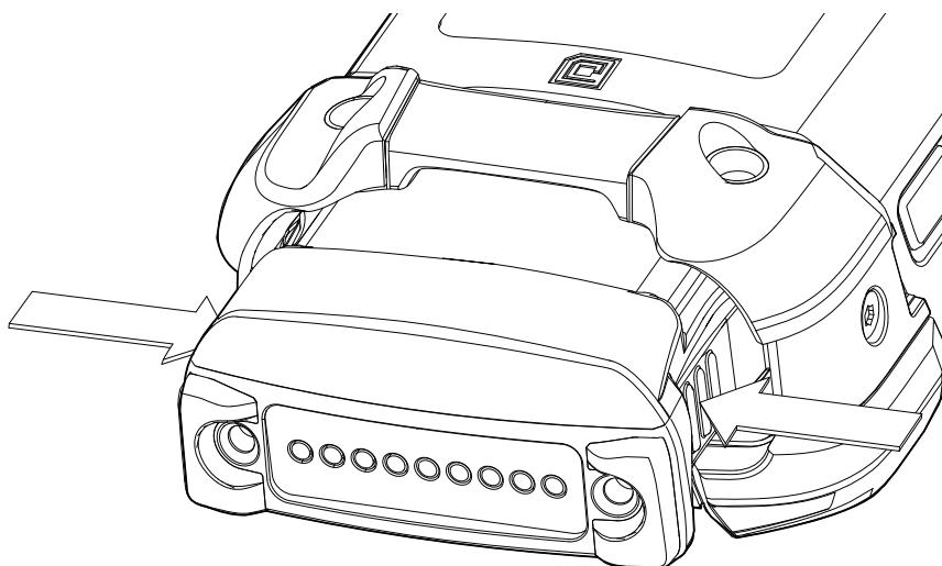
3. Remove the battery from the battery slot.
