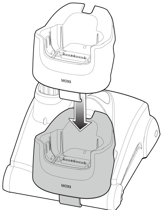
4. Insert the device into the cradle.
