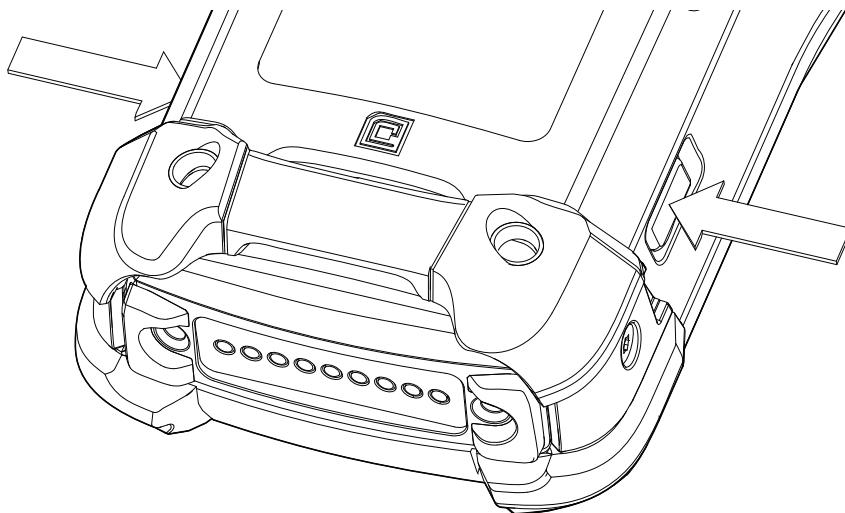
2. Push in the secondary battery release buttons on the sides of the battery.
