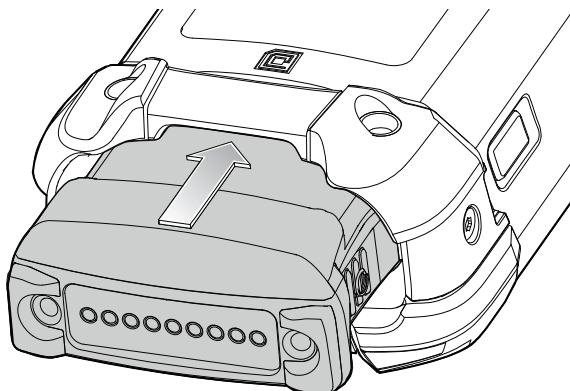
5. Push the battery into the battery slot.
