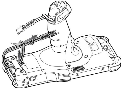
3. Attach the two plastic ends together.
