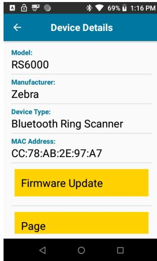
3. Under the RS6000 peripheral information, touch **Page** to page the RS6000. The paged RS6000 beeps and vibrates.
