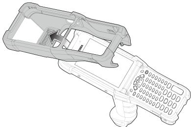
3. Grasp the bottom of the rubber boot and place over the bottom of the device.
