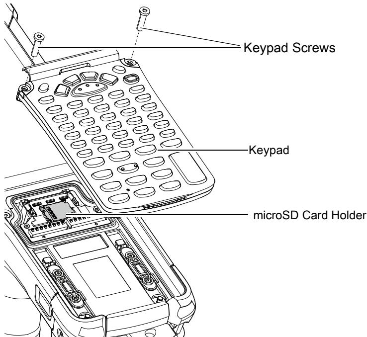
7. Lift the keypad from the device.
