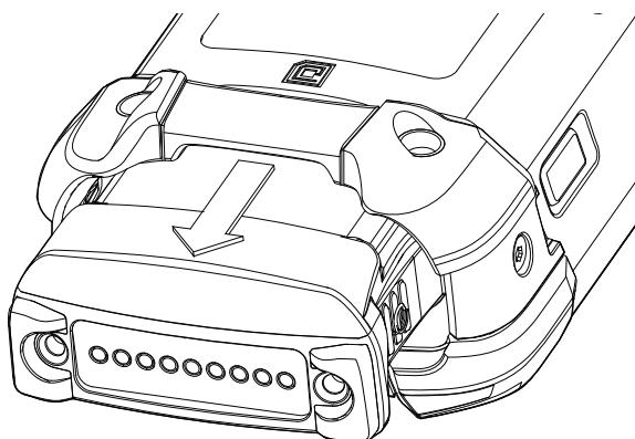
4. Align the battery with the battery slot.
