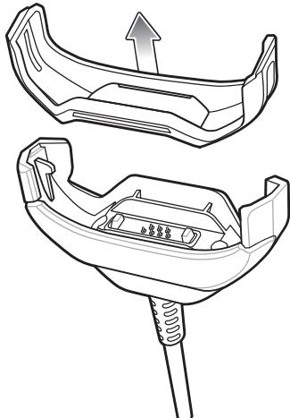
3. Align the cable cup with the bottom of the device.
