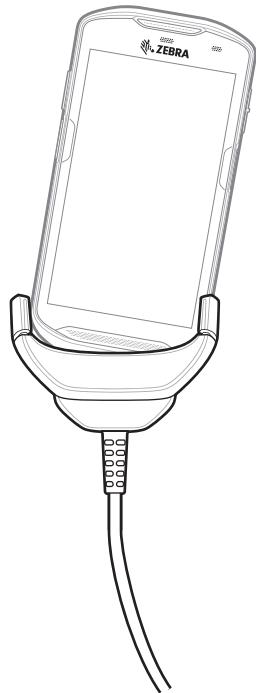
2. Rotate the device into the cup.
