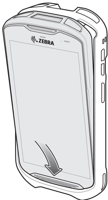
2. Lift the top of the Rugged Boot over the top of the device.
