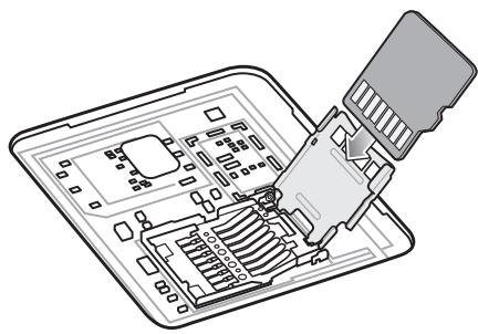
5. Close the microSD card holder and slide into the lock position.
