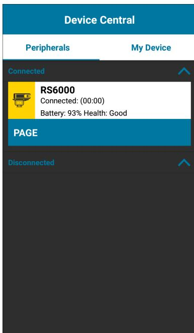
To stop paging, press the scan trigger of the RS6000. On a triggerless RS6000, reset the RS6000 to stop paging. Refer to the RS6000 User Guide.
