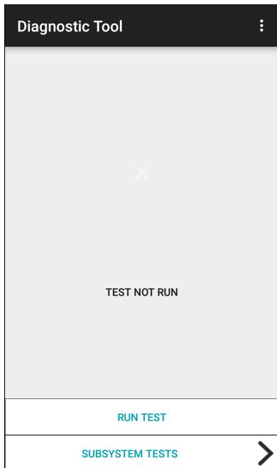
2. Touch **RUN TEST**. The app tests all enabled subsystems (by default, only the Battery and System tests). See [Settings on page 77](#) to enable subsystem tests.
