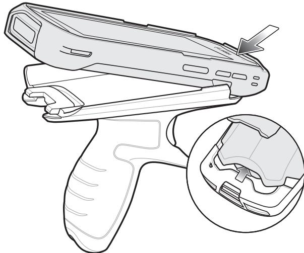
2. Rotate the device down and press down until it snaps into place.
