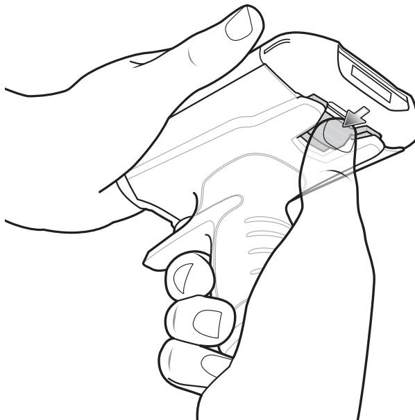
2. Slide the device forward and then rotate the bottom of the device up.
