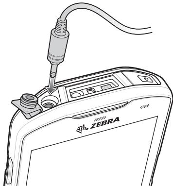
3. Connect the 3.5 mm connector plug of the headset into the 3.5 mm Audio Adapter.
