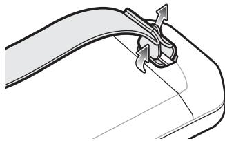
6. Align the hand strap clip with the top cap.
