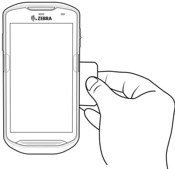
3. Move the device close to the NFC card until it detects the card.
