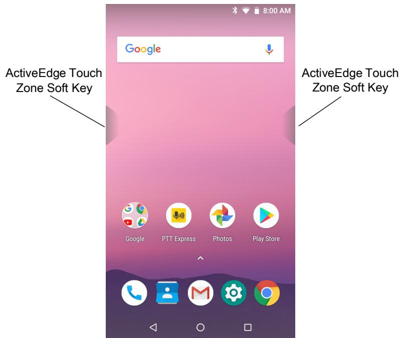
When a soft key is set to Scanner, touch and hold the soft key to scan a barcode.
