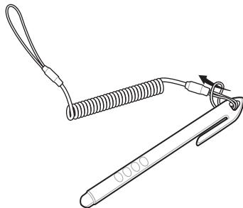
**Figure 136** Install Stylus on Hand Strap
