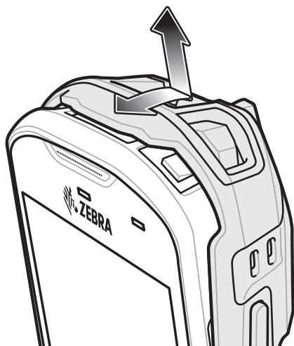
3. Push the device into the Rugged Boot.
