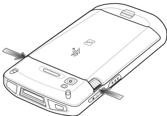
7. Lift the battery from the device.
