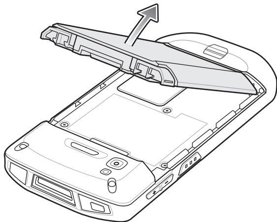
**CAUTION:** Replace the battery within 75 seconds. After 75 seconds the device reboots and data may be lost.
