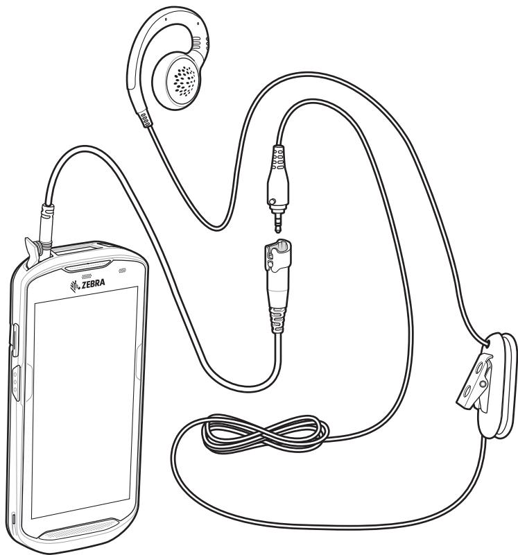
**CAUTION:** After removing headset, headset jack cover must be replaced and securely seated to ensure proper device sealing.
