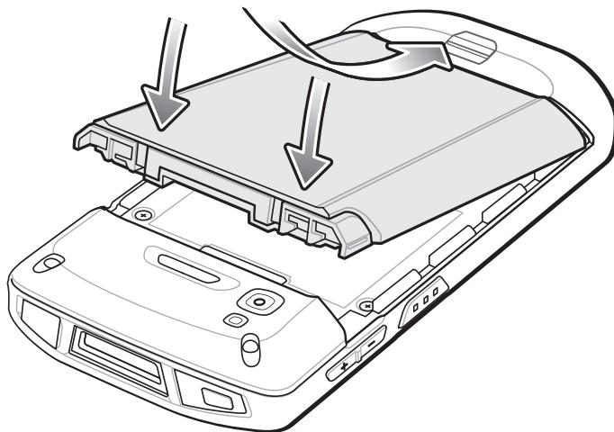
2. Press the battery down into the battery compartment until the battery release latches snap into place.
