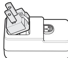
3. Insert the replace plug adapter into the power supply.
